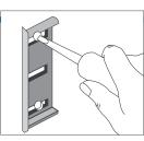
Remove end caps. Hold caps to corner markings and mark end cap mounting holes. Drill holes, insert anchors, and fasten caps to wall. do not fasten tightly; allow for minor adjustment.
